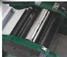
**Cutter Block** The three knife cutterblock ensures an excellent finish.
